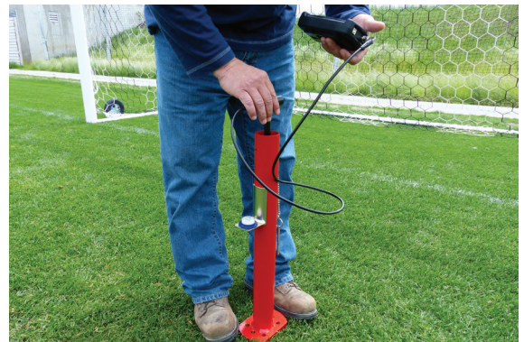
Greenhorizons measuring G-max ratings of the fields, 1 year post installation.
